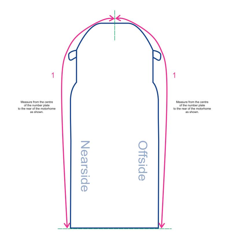
You only need to take measurements from one side of your vehicle 1 Rear of motorhome to the Centre of the front number plate =
